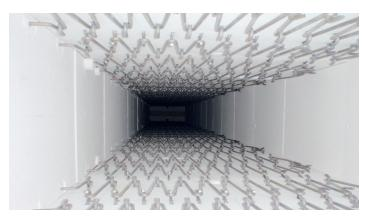
The expansion furnace is heated electrically only in vertically arranged heating zones.
