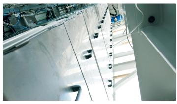
The desired quality of the final product determines the number of modules used in the expansion furnace. The system is adaptable and expandable to several modules and several parallel shaft furnaces.
